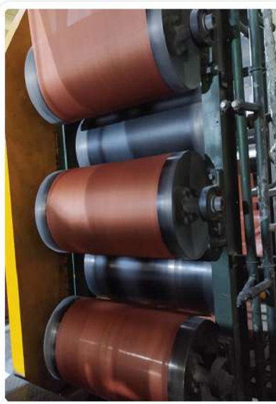
Calendering Nylon With Rubber
