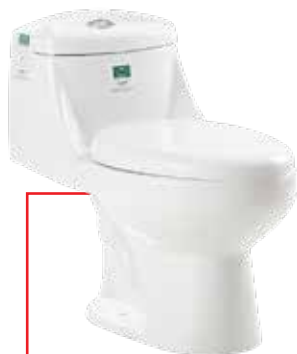
Commode One Pcs. AMT2088 Item code : 701939 (White) / 933567 (Ivory) Dimension : 720X380X650 mm Siphonic S-trap One Piece Closet
