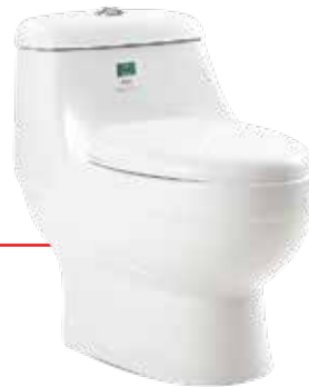
Commode One Pcs. AO002 Item code : 706053 (White) / 708004 (Ivory) Dimension : 715X410X715 mm Siphonic S-trap : 300 mm, Quick Release Seat Cover
